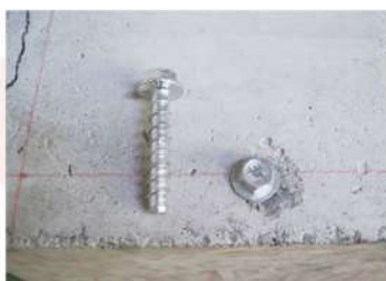
Self-Tapping Screw Anchor ✓ Perfectly Installed
