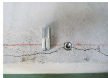
Drop-in Anchor ✗ Concrete Cracked
