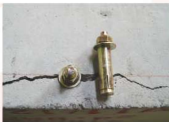
Expansion Anchor ✗ Concrete Cracked
