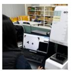
Incoming material/in-process inspection (Measured by the Vickers hardness test)
