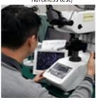
Incoming material/process/outgoing shipping inspection (Dimensional measurement with image tool microscope)
